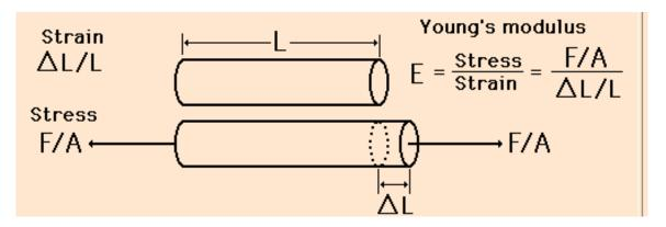
Like the bulk modulus, **Y** is defined in terms of stress/strain. Higher  $\mathbf{Y} \rightarrow$  harder to stretch. The units are again pressure units (e.g. pascals or N/m<sup>2</sup>). Numerically, the definition of Y is:
