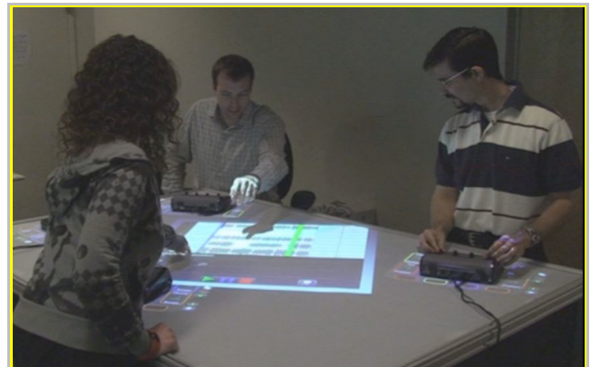
Figure 1: Dynamically re-mappable physical controllers are integrated into a multi-touch, collaborative tabletop environment.
